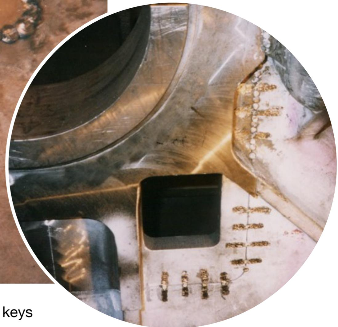
Apertures drilled off and filled with Metalock keys
