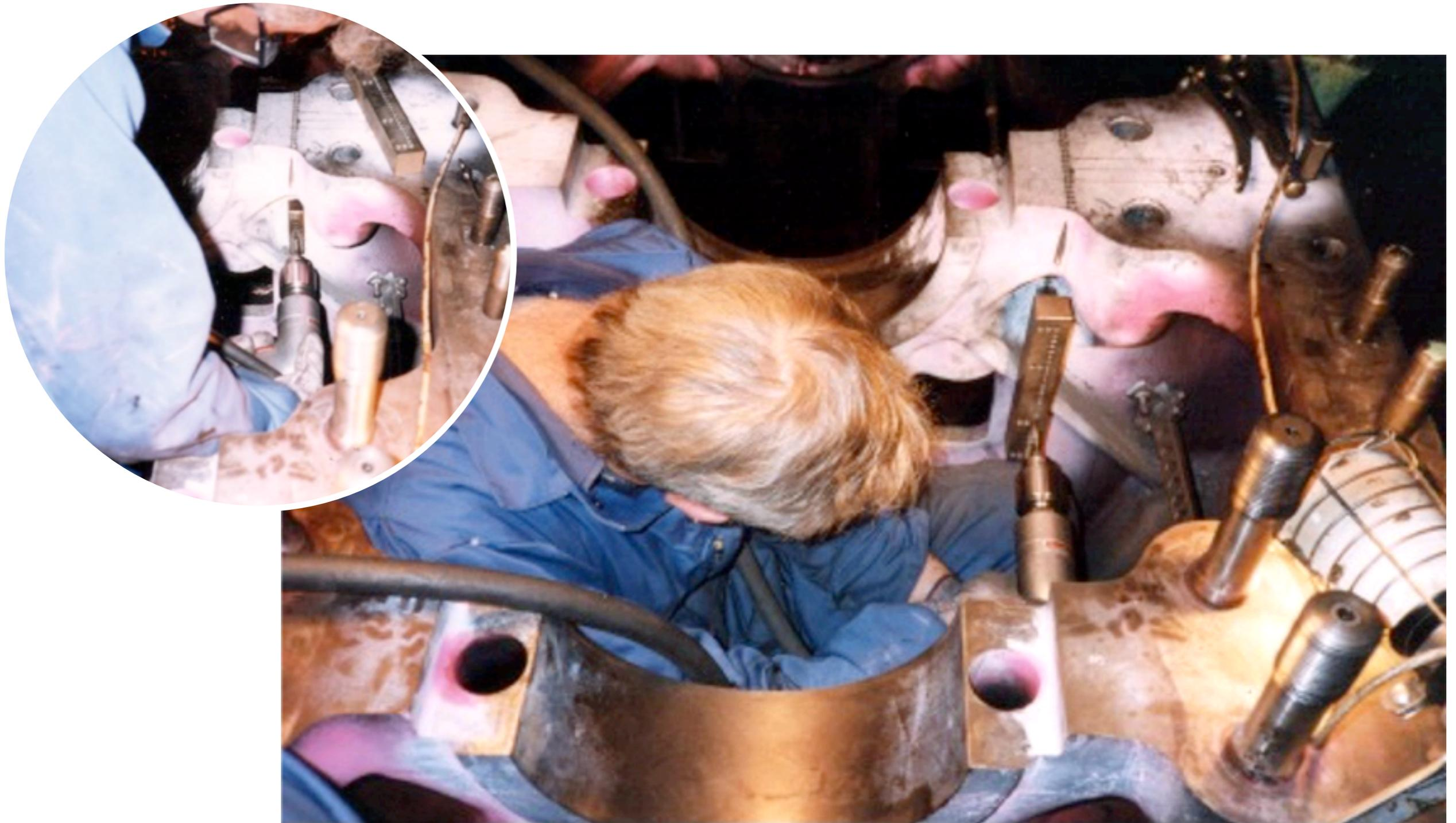
The drilling was through the full depth of the parent casting
