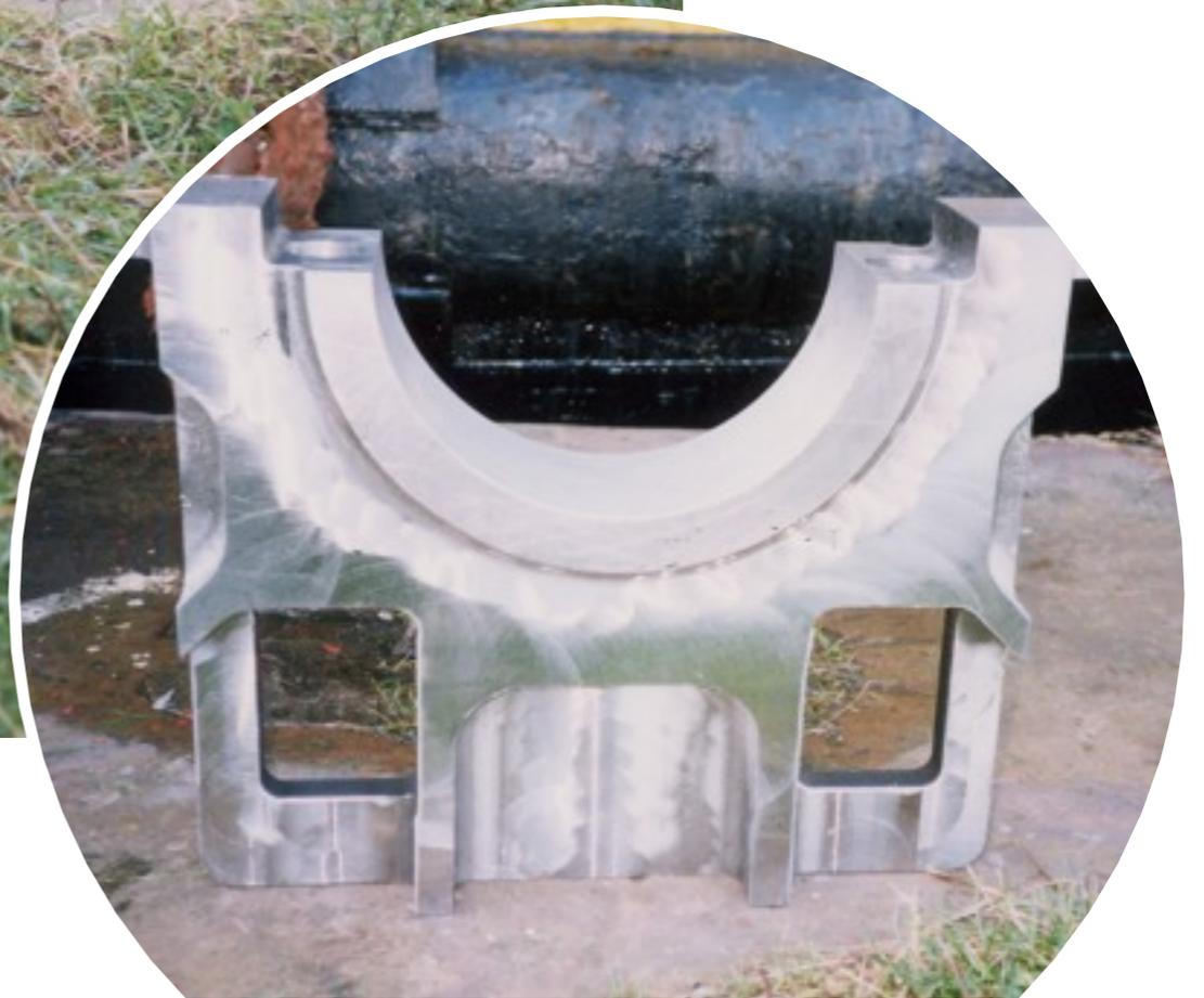
Insert showing attached Masterlocks to help spread the load
